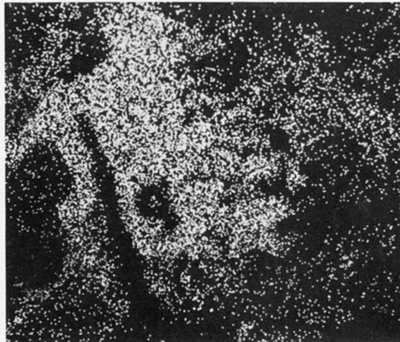
FIGURE 11. Electron microprobe images illustrating occurrence of leucite (high K and low Na concentrations) in basanite P90: top, back-scattered electron image; bottom left, K distribution; bottom right, Na distribution.
